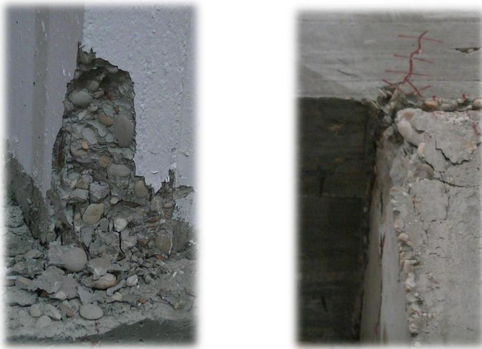
**Figure (11):** Localized Damage and Crack Development Observed towards the End of the ENEA Shake Table Tests
