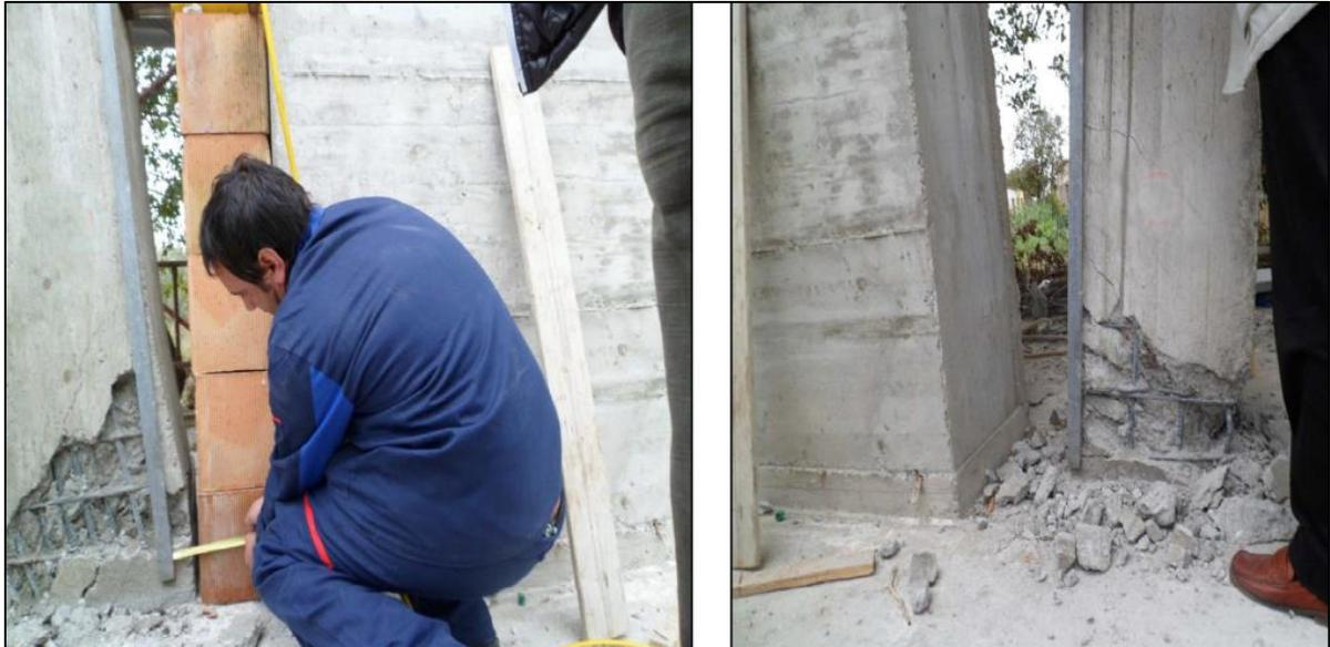
**Figure (12):** Comparison between The Conventional (without core) and the Column Specimen with the Pillar Bone Core System
