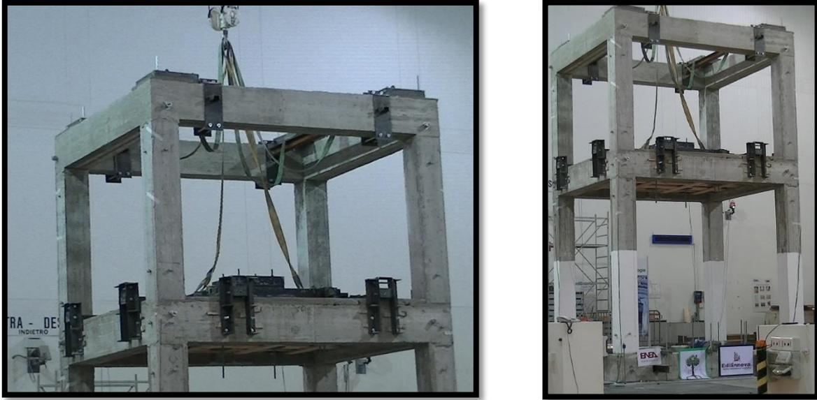
**Figure (4):** Typical 2-Story Reinforced Concrete Frame Structure Specimens
