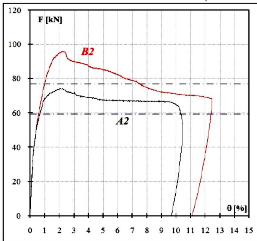
**Figure (13):** Large-Scale Experimental Results from University of Naples Shown the Higher Strength and Ductility of Column “B2” with the Pillar Bone Core System as Compared to the Conventional Column “A2”
