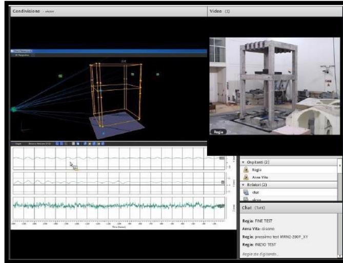
**Figure (6): Remote Witnessing via Internet for about 200 Users Using DySCo Virtual Laboratory (Building Model “B”)**
