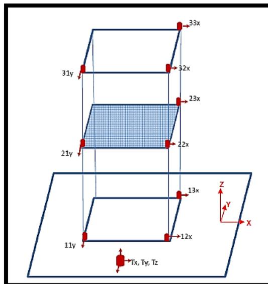
**Figure (5):** Typical Electronic Accelerometers Locations
