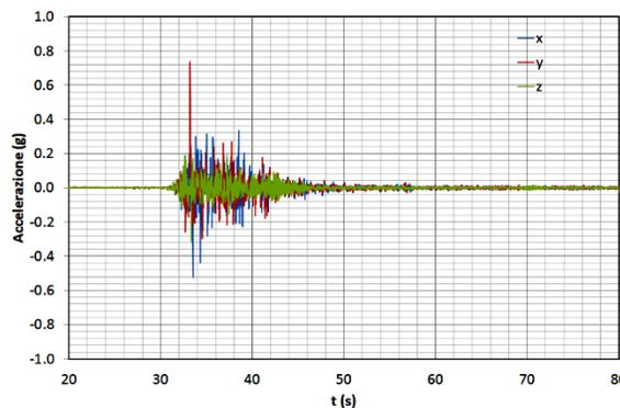
**Figure (9):** A Sample of Seismic Input used for the Three Model Buildings Tests
