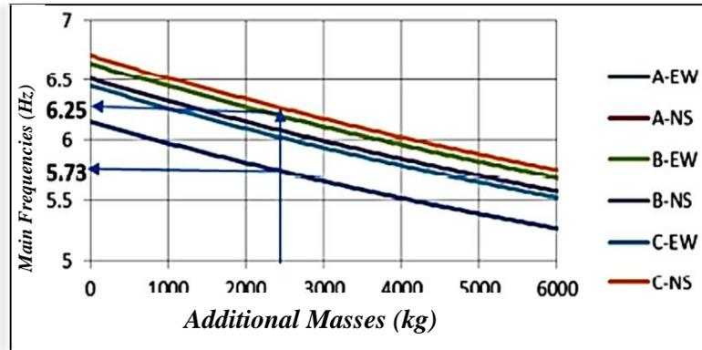
**Figure (8):** Estimate of Main Frequencies in E-W and N-S Directions vs. Additional Masses for the Three Model Buildings (A, B, and C)
