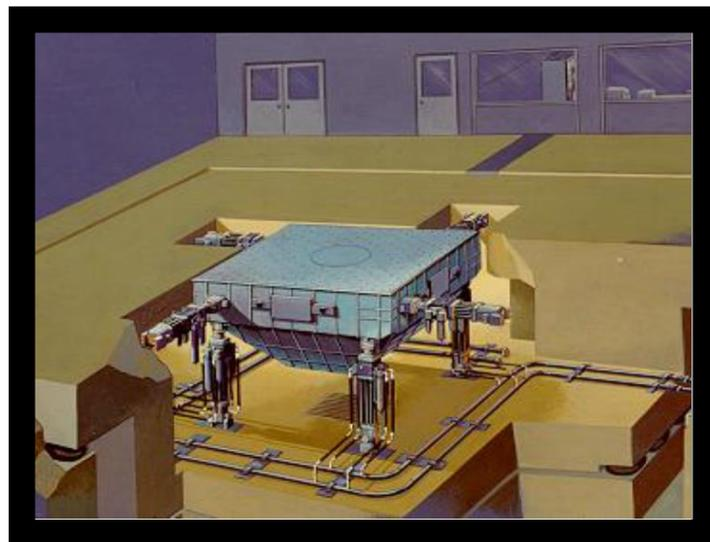
**Figure (7): Schematic Section of the 4.0 m X 4.0 m a 6GDL Shake Table used in Evaluating EDILINNOVA Innovative Pillar Bone Rehabilitation Technology**
