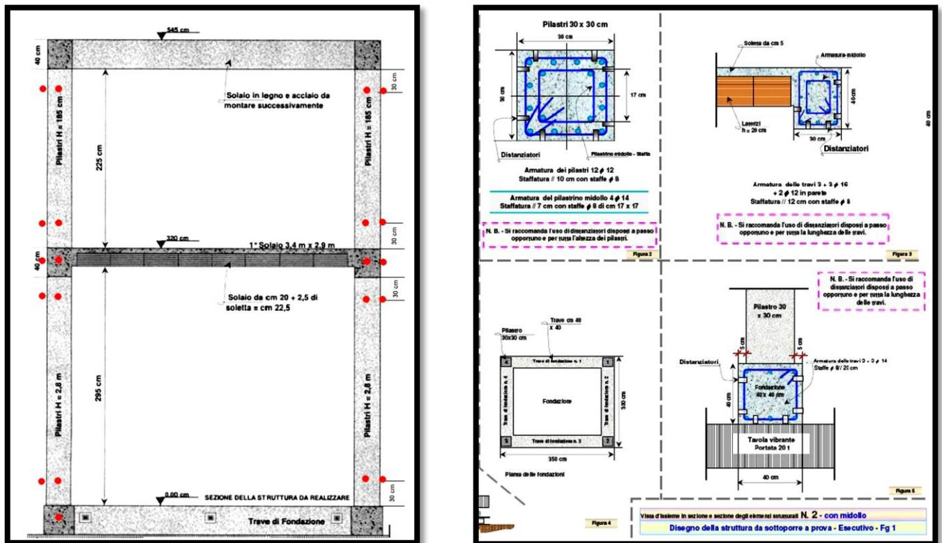
**Figure (3):** Typical Dimensions and Geometry of 2-Story Frame Structure Specimens
